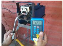
Pyrometer indicating proper blade temperature of 650°C.
